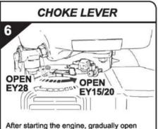
After starting the engine, gradually open choke by turning the choke lever and finally keep it open fully.
