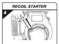
Pull the starter handle slowly and return the handle to its original position when resistance is felt.
