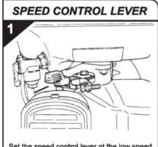
Set the speed control lever at the low speed position (L) and allow the engine to run at low speed for 1 or 2 minutes before stopping.
